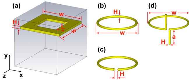
FIG. 1. (Color online) Schematic of the structures under investigation;  $w = 2.75 \mu\text{m}$ ,  $H = 0.15 \mu\text{m}$ ,  $L = 0.055\text{--}1.375 \mu\text{m}$ , and  $a = 0\text{--}1.125 \mu\text{m}$ , respectively. In (a) one can notice the  $3 \times 3 \times 3 \mu\text{m}^3$  metallic cavity, in which each of the studied structures are embedded, close to its top surface.
