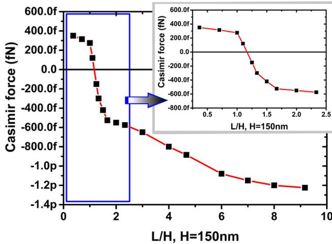
FIG. 3. (Color online) Casimir force along the  $y$  axis at a distance  $d = 300$  nm between the top surface of the cavity and the proposed structure of Fig. 1(a) as a function of the ratio  $L/H$ . In the inset, one can see a more detailed presentation of the Casimir force for  $L/H = 0.25$ – $2.5$ .
