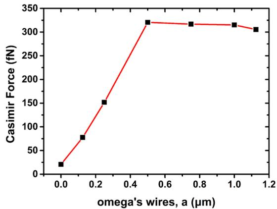
FIG. 5. (Color online) Repulsive Casimir force of the proposed “omega” particle embedded into a  $3 \times 3 \times 3 \mu\text{m}^3$  cavity, as a function of its wire’s length  $a$ . For these types of calculations, as opposed to the one shown in Fig. 4, the loop of the “omega” particle was placed at a symmetric position in the  $3 \times 3 \times 3 \mu\text{m}^3$  cavity, and several cases of wires were studied with length  $a = 0.0\text{--}1.125 \mu\text{m}$ .
