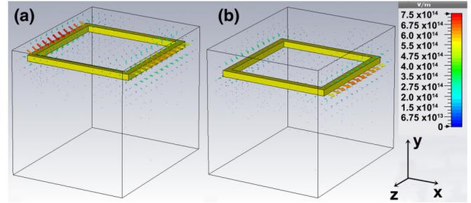
FIG. 2. (Color online) The  $3 \times 3 \times 3 \mu\text{m}^3$  boundary box acting as a metallic cavity with the metallic structure (with  $L = 0.150 \mu\text{m}$ ) embedded into it. The distance of the structure from the top surface of the boundary box is (a) 100 and (b) 500 nm, respectively. A snapshot of the electric field distribution on the metallic structure embedded into the  $3 \times 3 \times 3 \mu\text{m}^3$  boundary box is shown.
