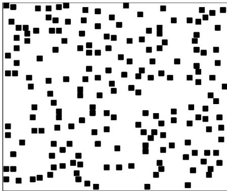
FIG. 1. Typical sample configuration. The size of the system is  $128 \times 128$ , the filling factor  $x=0.1$ . 182 rectangular rods with square cross section of  $3 \times 3$  are randomly distributed throughout the sample. Scalar wave propagates from left to the right.
