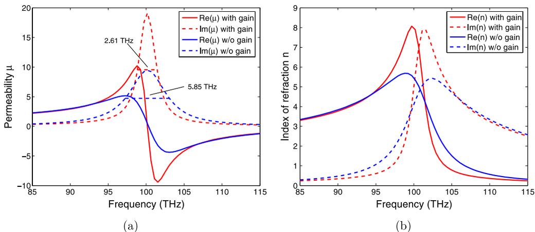
**Figure 18.** The retrieved results for the real and the imaginary parts of (a) the effective permeability  $\mu$  and (b) the corresponding effective index of refraction  $n$ , with and without gain for a pumping rate  $\Gamma_{\text{pump}} = 1.0 \times 10^9 \text{ s}^{-1}$  and the SRR system of figure 17. The gain bandwidth is 20 THz. Notice that the width of the magnetic resonance with gain is 2.61 THz.
