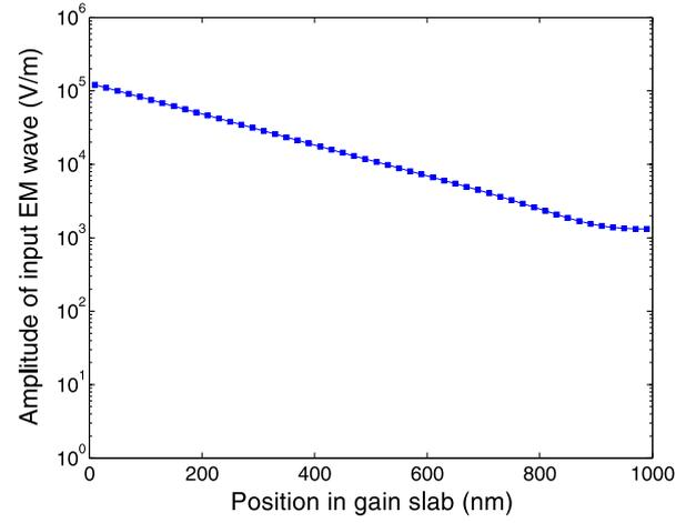
**Figure 6.** The amplitude of the input EM wave inside the gain slab as a function of the position. The gain slab width  $w = 1000$  nm and the input power  $P_{in} = 92.3$  W mm<sup>-2</sup>. All other parameters are the same as figure 3.
