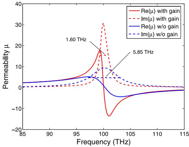
**Figure 19.** The retrieved results for the real and the imaginary parts of the effective permeability,  $\mu$ , with and without gain for a pumping rate  $\Gamma_{\text{pump}} = 8.0 \times 10^8 \text{ s}^{-1}$  and the SRR system where the SRR is surrounded by gain. The gain bandwidth is 20 THz. Notice that the width of the magnetic resonance with gain is 1.60 THz, narrower than figure 18(a).
