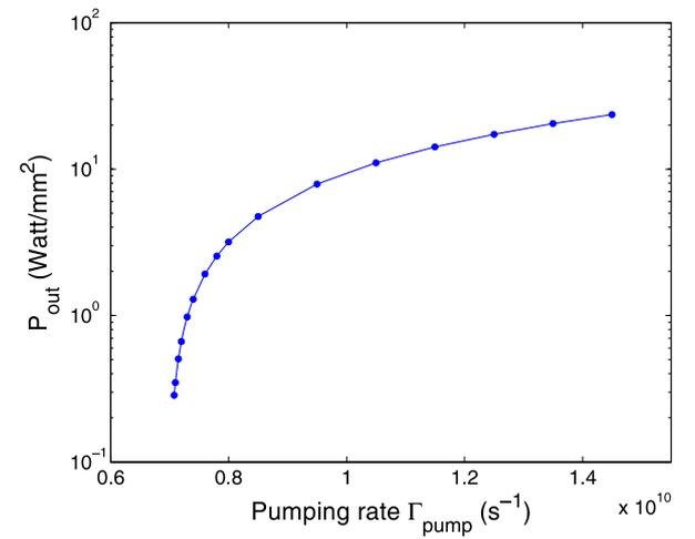
**Figure 7.** The powers emitted at the emission frequency  $\omega = \omega_a$  (100 THz) for different pumping rates. The gain slab width  $w = 100$  nm and the bandwidth of the atomic transition between  $N_1$  and  $N_2$  is 5 THz.
