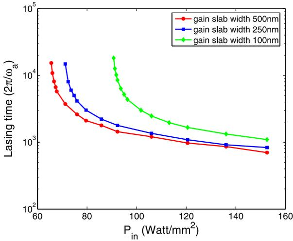
**Figure 5.** The lasing times for different input powers at the pumping frequency  $\omega_b$  (200 THz). The gain slab width  $w = 100$  nm, 250 nm and 500 nm, respectively. All other parameters are the same as figure 3.
