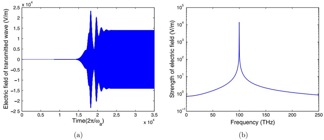
**Figure 14.** (a) The time-dependent electric field of the transmitted wave for a three-layer system (NIM—gain material—NIM) and (b) the corresponding Fourier transform in frequency domain for the lasing in (a). The pumping rate  $\Gamma_{\text{pump}} = 1.5 \times 10^{10} \text{ s}^{-1}$ .
