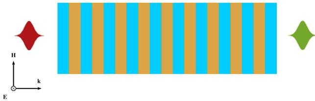
**Figure 9.** The negative index material (blue) embedded in layers of gain material (orange). The number of layers, the permittivity and permeability of NIM take different values for the different cases we have examined. The width for both NIM and gain material is  $w = 50$  nm. The gain bandwidth is 5 THz.
