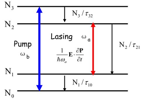
Figure 1. Schematic of the four-level atomic system model.
