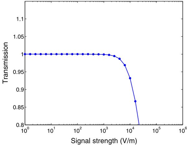
**Figure 11.** The transmission versus signal amplitude for the loss-compensated metamaterial of figure 9 with a gain bandwidth of 5 THz at the critical pumping rate  $\Gamma_{\text{pump}} = 1.98 \times 10^9 \text{ s}^{-1}$ . The material parameters for the NIM are same as figure 10. For incident fields stronger than  $10^3 \text{ V m}^{-1}$  this metamaterial becomes nonlinear.
