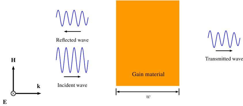
**Figure 2.** Schematic of gain material slab (shown in orange). The slab width  $w$  takes different values in the cases we have examined.
