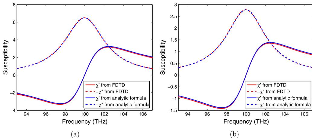
**Figure 13.** The numerical and analytical results for the susceptibilities of gain materials as a function of frequency. (a) A three-layer system (NIM—gain material—NIM) at the critical pumping rate  $\Gamma_{\text{pump}} = 4.7 \times 10^9 \text{ s}^{-1}$ . (b) A 19-layer system of figure 9 at the critical pumping rate  $\Gamma_{\text{pump}} = 1.98 \times 10^9 \text{ s}^{-1}$ .
