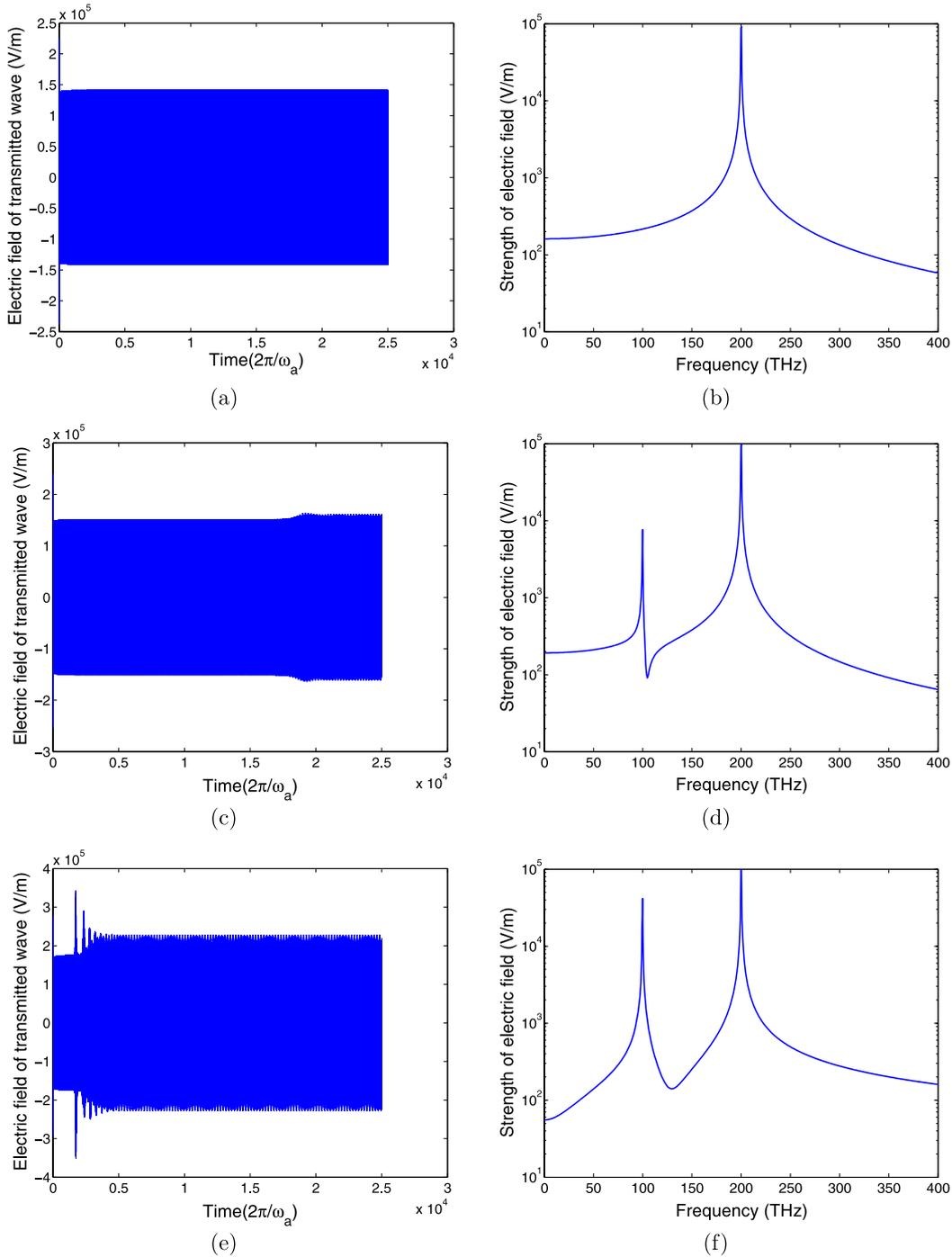
**Figure 3.** The transmitted waves and their corresponding Fourier transforms for different input powers. (a), (c) and (e) are the transmitted waves for input power  $P_{in} = 79.6, 90.7$  and  $120.6$  W mm<sup>-2</sup>, respectively. (b), (d) and (f) are same as (a), (c) and (e), respectively, but are the Fourier transforms of the transmitted waves. The gain slab width  $w = 100$  nm and the bandwidth  $\Gamma_a$  of the atomic transition between  $N_1$  and  $N_2$  is 5 THz.
