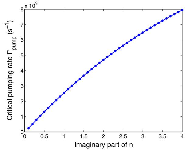
**Figure 12.** The critical pumping rates for different imaginary parts of the refractive index  $n$  of NIMs. The structure is a three-layer system (NIM—gain material—NIM) and  $\epsilon = \mu$  for NIMs.
